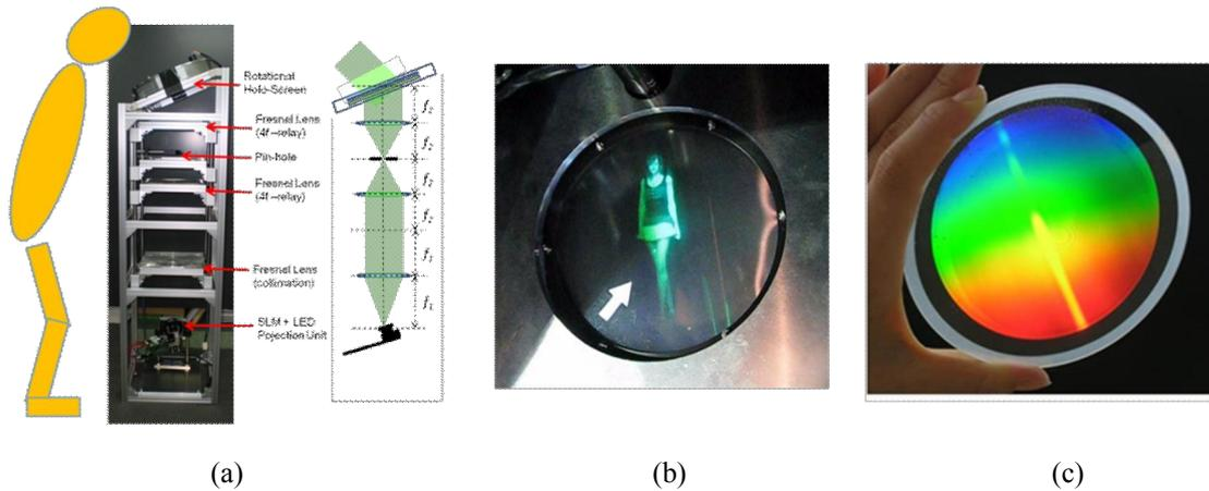
Fig. 1: Direct Light Scanning 3-D Display System Prototype. (a) System configuration of prototype (b) Displayed 3-D motion image (c) Holographic screen made by photopolymer material.
