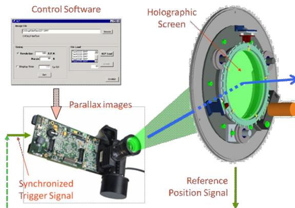
Fig. 3: System diagram of 3-D display prototype.
