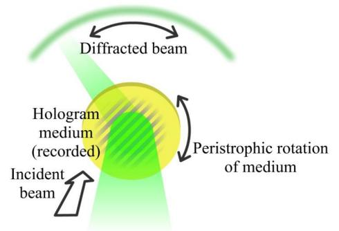
Fig. 2: Beam scanning by peristrophic rotation of holographic screen.
