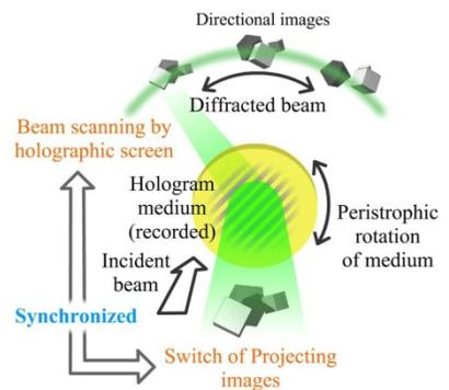
Fig. 3 Beam scanning by rotation of hologram screen.
