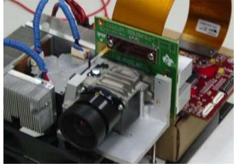
Fig. 4 Developed RGB display engine.
